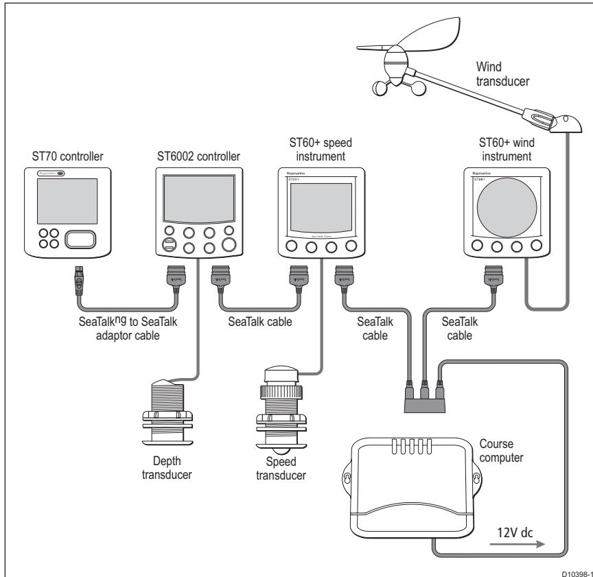
**Note:** You cannot calibrate an S1, S2 or S3 SmartPilot computer with an ST70 autopilot controller, you must use a SmartPilot controller.
