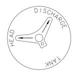
LEVER SET IN THIS POSITION FOR OVERBOARD DISCHARGE
