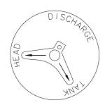
LEVER SET IN THIS POSITION FOR TANK DISCHARGE
