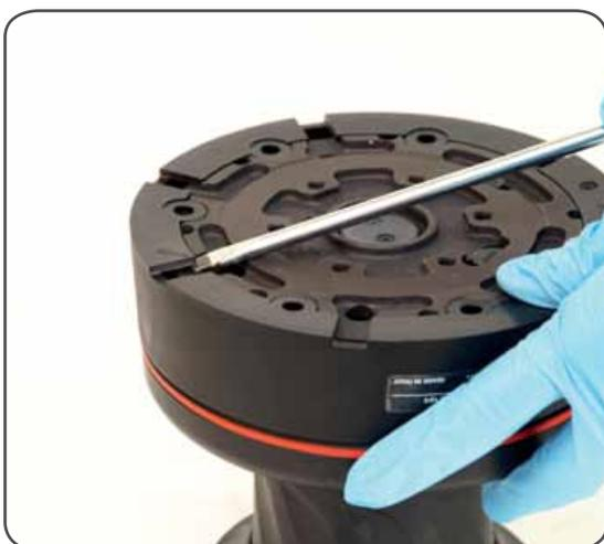
1. Remove the skirt n°2 with the help of the screwdriver placed as shown by the symbol
