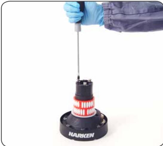
6. Completely unscrew the three screws n° 27
